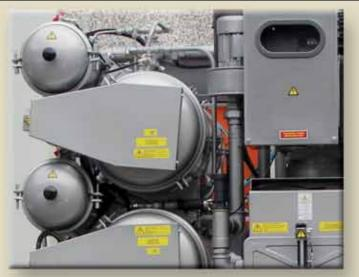
Multiple, independently functioning high-micron self-cleaning spin disc EcoFilters® and large-capacity carbon cartridge filters are available on all Union K Series Systems to assure optimum filtration of both large and small particles for maximum solvent purity. Computer controls automatically pair filter operation for whites, darks or colors according to specific pro-
